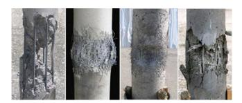
Safety: Polymer concrete, an energy-absorbing material against blast loads. © Fraunhofer EMI PRESS RELEASE
