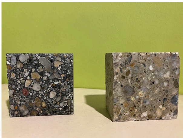
Fig. 1 Concrete with and without pyrochar: One part pyrochar can reduce three parts CO 2 in the final product.
